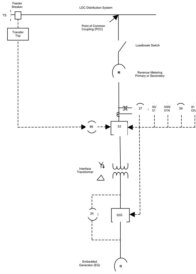
**Figure 2** Typical Single-Line Diagram Required at the Design Review Stage
