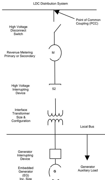
**Figure 1** Typical Single Line Diagram Required at the Connection Impact Assessment Stage
