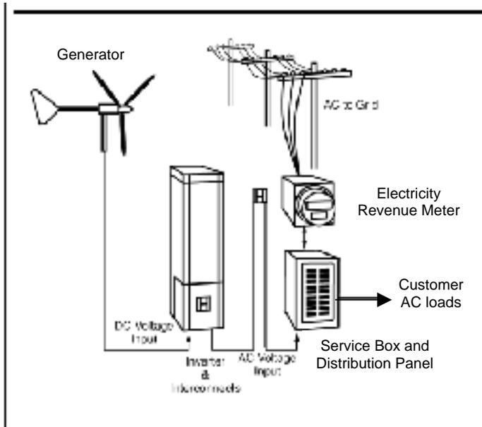
**FIGURE 1.** Diagram of a grid-tied wind electric system with “DG system disconnect”
